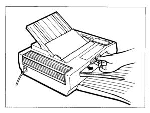
Grasp the jammed document firmly on both edges and pull it back to the rear. Make sure any small pieces of document which may have torn off are removed, use tweezers if necessary.
